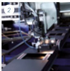
2. Automatic loading station of an in-line PE-CVD deposition system for anti reflective and passivation coatings on c-Si solar cells ©SINGULUS TECHNOLOGIES AG
