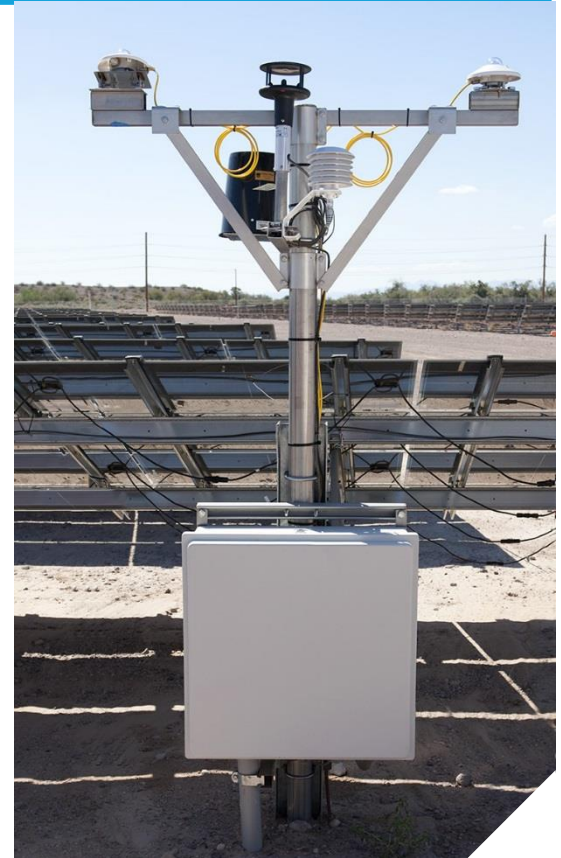
Field Weather Station
