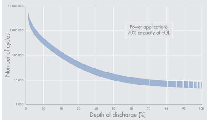
*Cycle life depends on both depth of discharge (DOD) and charging rates. The above results are based on testing at a fixed DOD and varying charging rates. The end of life (EOL) is reached when the remaining capacity is 70% of the initial capacity.*
