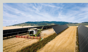
(c) Interspace PV with clearance
